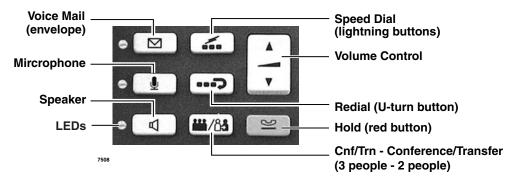
**Note** The IPT Fixed Buttons work the same way as the DKT telephones, however on the IPTs, fixed buttons have been replaced with button icons.
