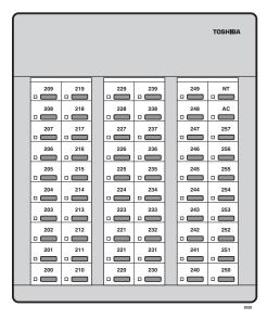
The DDSS3060 console uses dual red and green LEDs to show call and feature status.
